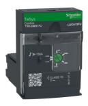
Standard control unit, TeSys Ultra, 3P, 3 to 12A, 690VAC, thermal magnetic protection, class 10, 110 to 240VAC/DC coil
